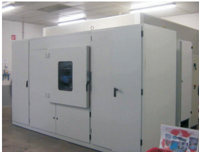
Acoustic chamber for compressor
