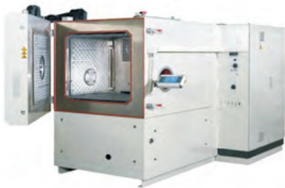
Vacuum Chamber fitted with shrouds
