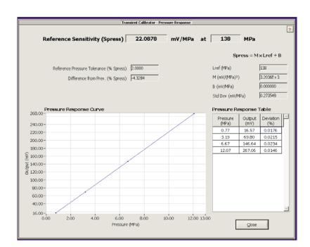
K9907C calibrates at pre-determined levels and calculates linearity over the testing range
