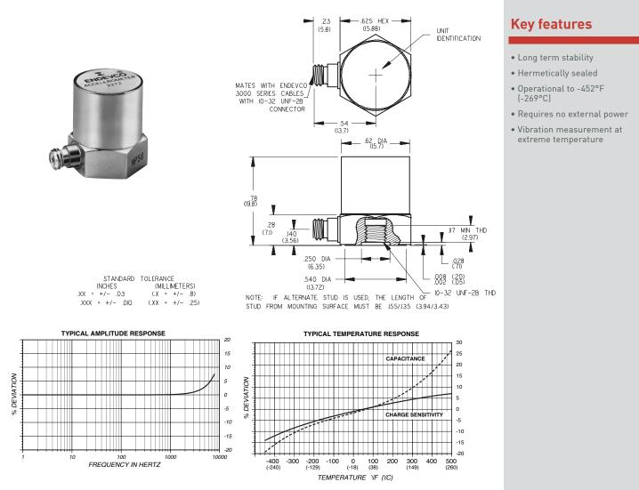
The Endevco® model 2272 is a piezoelectric accelerometer designed specifically for vibration measurement at temperature extremes. The unit is hermetically sealed for use in harsh environments and features long term stability. Its unique sensing elements offer an unusually flat temperature response over a broad range. The accelerometer is a self-generating device that requires no external power source for operation.
