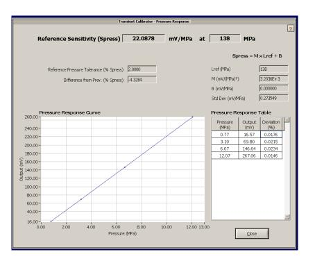
K9905D calibrates at pre-determined levels and calculates linearity over the testing range
