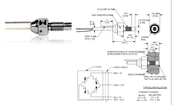
Model 8510B is a rugged, miniature, high sensitivity piezoresistive pressure transducer. It has a 10-32 mounting thread, 0.15 inch (3.8 mm) face diameter and is available in ranges from 1 psi to 2000 psi. Low pressure ranges are shown on this sheet. Its high sensitivity combined with high resonance makes it ideal for measuring dynamic pressure.
