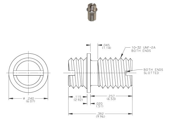
Mounting stud with slotted head for use with accelerometers with a 10-32 thread.
