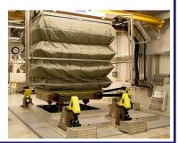
**Chamber Equipment:** Bellows, (H 2565 x W 2750 x D 3270 mm) 2 zippers, 2 DN100 ports for measuring cables.
