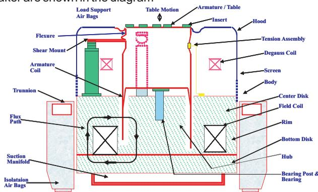
The field coils energize the shaker body with flux paths as shown, creating a high magnetic flux density in the annular air gap. The field coils are connected to the DC field supply. The armature assembly, consisting of the table and the driver coil, is suspended in the annular air gap of the shaker. When an alternating current is passed through the driver coil, electrodynamic forces are generated on the driver coil wire causing the table to move up and down.
