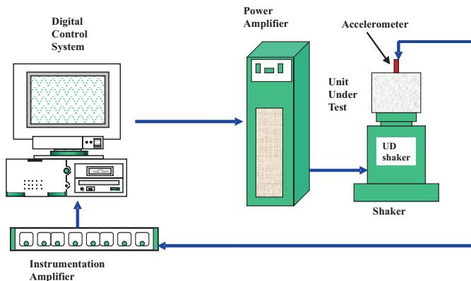
The Diagram above represents a typical vibration test system. A vibration test system is comprised of: An Electro dynamic shaker, A Power Amplifier, Digital Control System and support instrumentation. Together these items form a complete "closed loop" system that can accurately reproduce a defined vibration environment.
