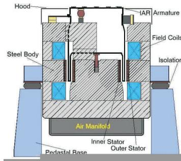
Through transformer coupling, AC currents flow in the single turn secondary. Field coils in the shaker generate a concentrated DC magnetic field in the air gap where the armature is suspended. The current in the armature ring reacts with the magnetic field generating a force on the moving element. This interaction generates AC forces on the INDUCT-A-RING, thus causing motion of the armature
