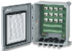
Model 691A50/12 BNC Termination Box ● For use with data collectors that supply ICP sensor power ● 12 input channels via terminal strip ● 12 output channels via BNC's ● NEMA-4X (IP66) enclosure
