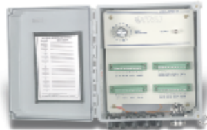
Model 691B47 Rotary Switch Box ● For use with data collectors that supply ICP sensor power ● 16 input channels via terminal strip ● BNC output connector for switched vibration signal ● NEMA-4X (IP66) enclosure
