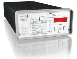
Endevco® model 136 is a three-channel, DC amplifier that is manually or computer programmable. Manual control is accomplished at the front panel by means of a "select channel" push-button, three (3) "channel LEDs", one "select function" push-button, five "function LEDs", a four character LED display, showing the state of each function/channel, and four "edit" push-buttons to change the entries in the LED display. There are three LEDs used as fault status indicators for the auto zero function.
