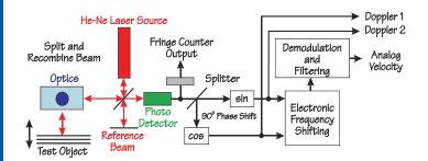
The intensity of recombined beam is modulated according to F=v/( $\frac{1}{2}$ )where F<sub>a</sub>=Doppler frequency v=test object velocity
