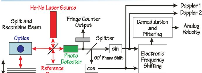
The intensity of recombined beam is modulated according to  $F = v / (\lambda/2)$  where
