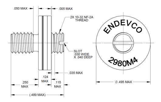
Isolated mounting adapter with .495 inch diameter for use with accelerometers with a 10-32 thread.
