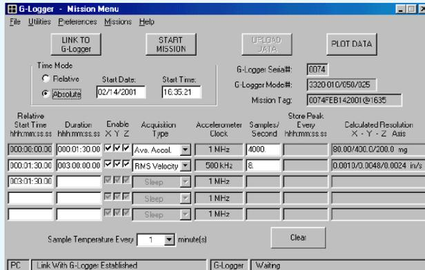
RS-232 COM port. The G-Logger Software program is meant to be used in conjunction with the optional EasyPlot data graphing and plotting program. Should you already own or choose to provide your own plotting software, the G-Logger Software Program can be set to output the data in an ASCII comma delimited format which is readable by most data graphing software packages.
