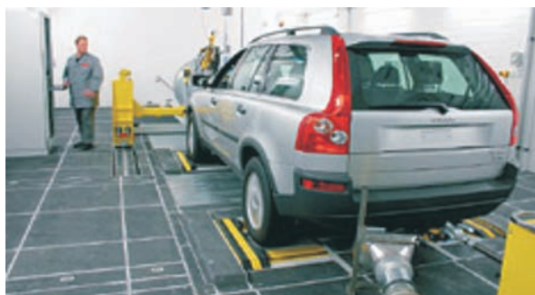
48" Emission Chassis Dyno (motor-in-the-middle principle) for rear-, front- and/or 4WD-vehicles
