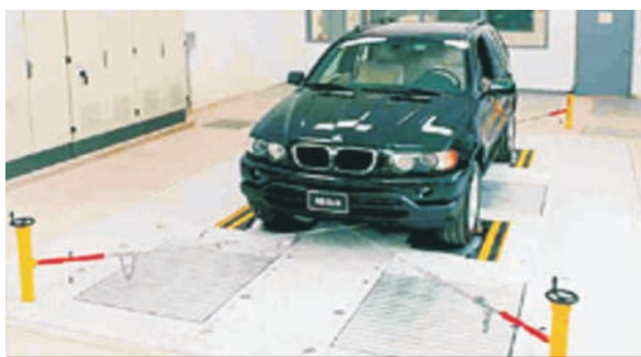
20" Emission Chassis Dyno (double rollers) for rear-, front- and 4WD Vehicles
